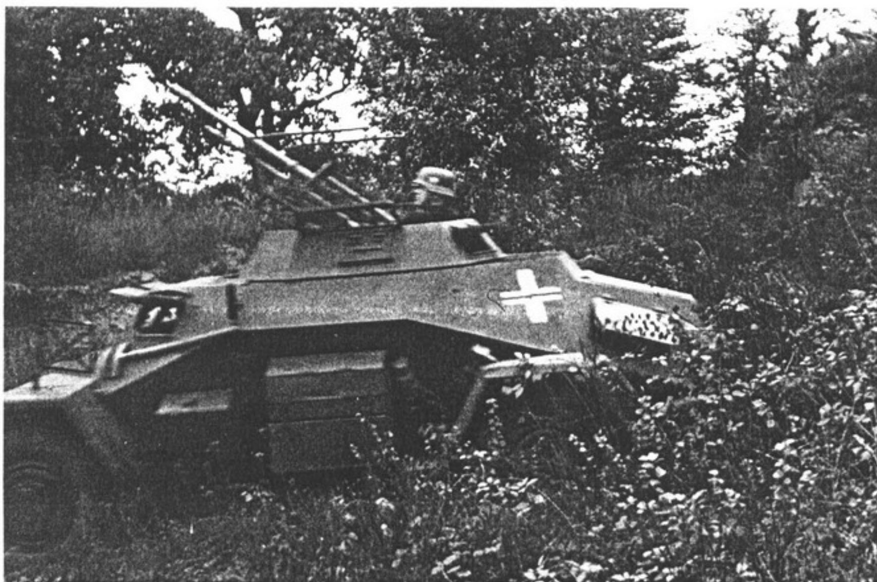
Left: The mount for the 20 mm gun in the le.Pz.Sp.Wg. (2 cm) (Sd.Kfz.222) was designed for the dual role of engaging aircraft and ground targets. (BA 58/1785/23)
