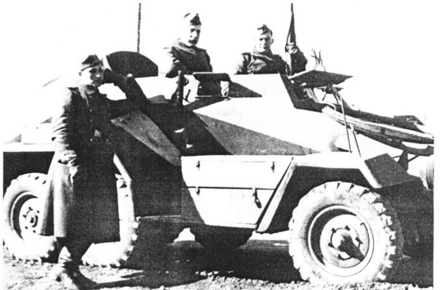
Right: This 6-wheel armored staff car was built on a Krupp L2H143 chassis (GF)
