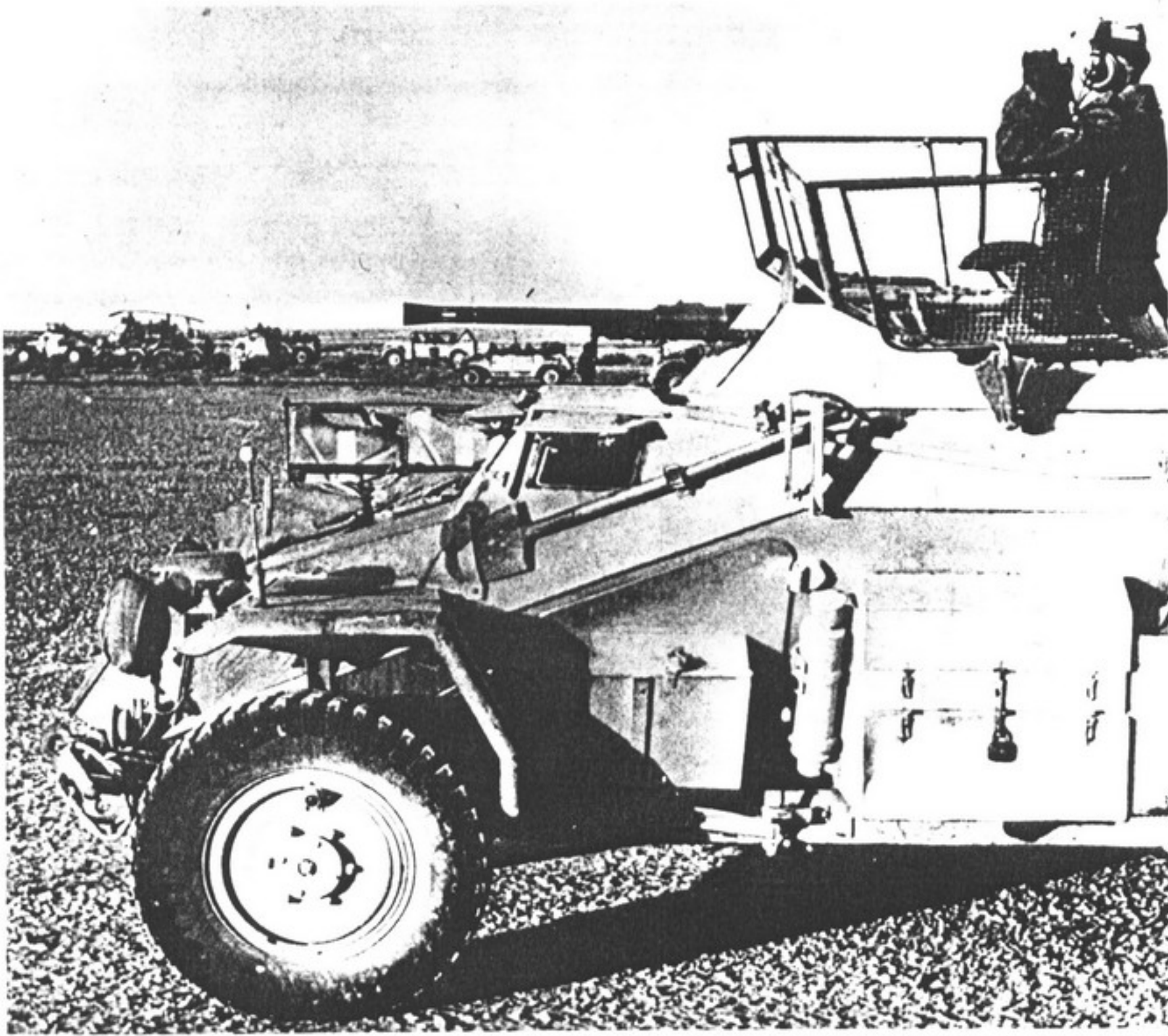
Left: A le.Pz.Sp.Wg. (2 cm) (Sd.Kfz.222) with Rommel's forces in North Africa (APG)
