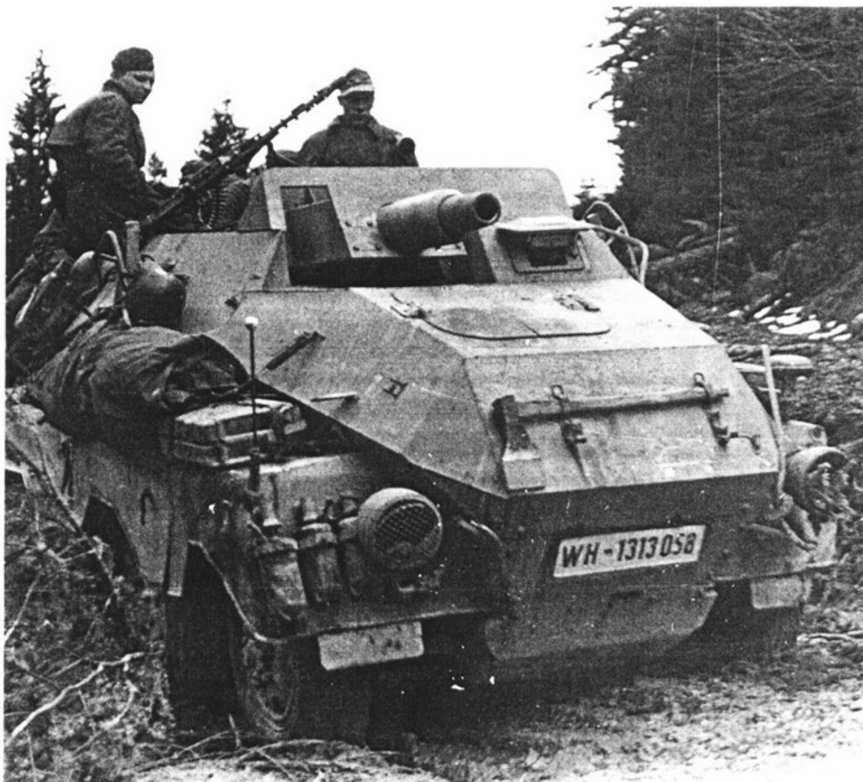
Right: A Sd.Kfz.233 in service in Russia with a M.G.42 on a pivoting mount (BA 205/1800/34a)
