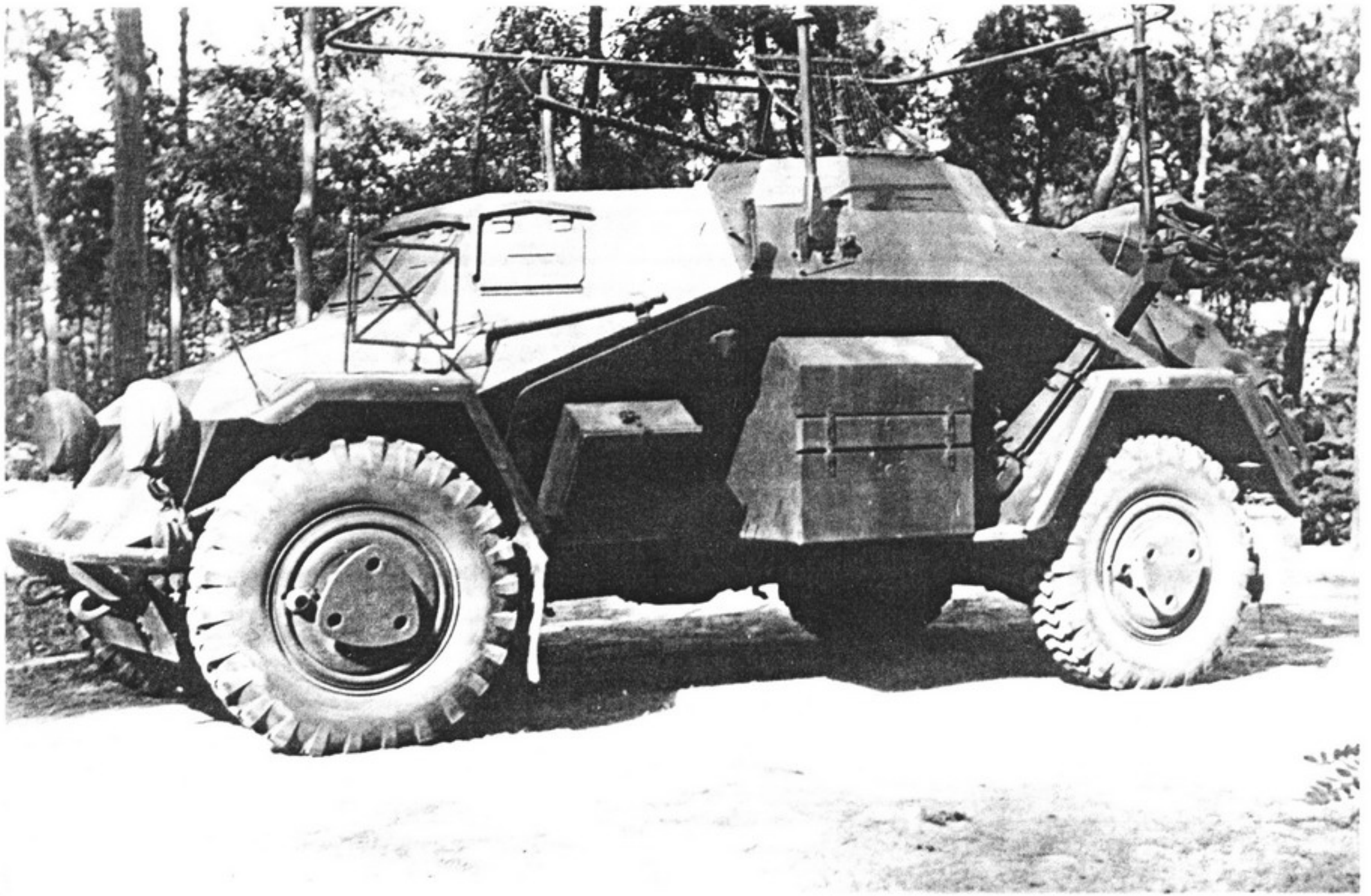
Above: One of the first production series Sd.Kfz.223 (Fgst.Nr.810338) was sold to China. (TTM)
