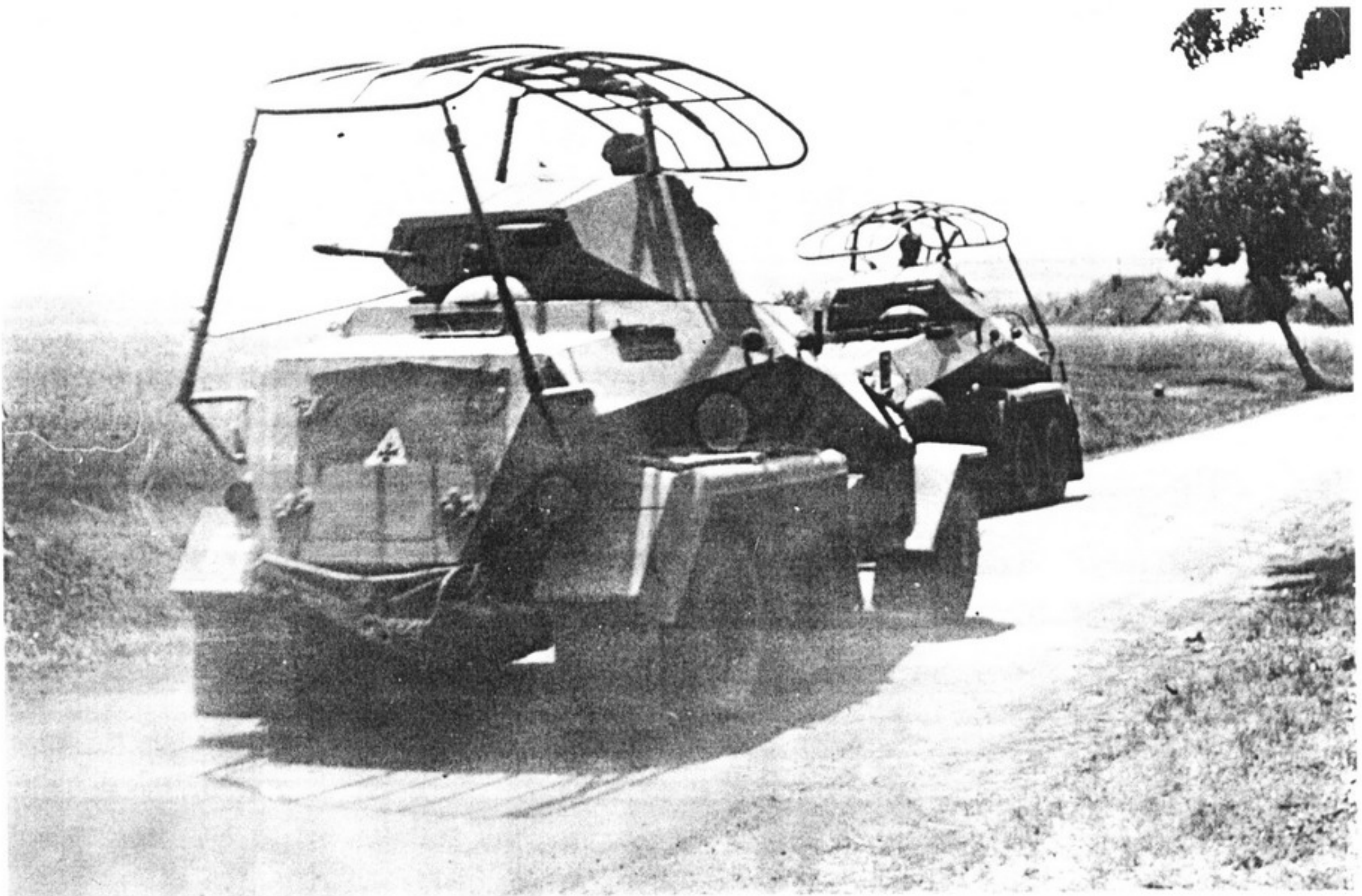
Above: S.Pz.Sp.Wg. (Sd.Kfz.231) were modified to mount an anti-aircraft machinegun on the turret with an external seat for the commander. (WJS) Below: A s.Pz.Sp.Wg. (Fu) (Sd.Kfz.232) on maneuvers in the Summer of 1935 before being modified to carry a spare tire on the rear. (APG)
