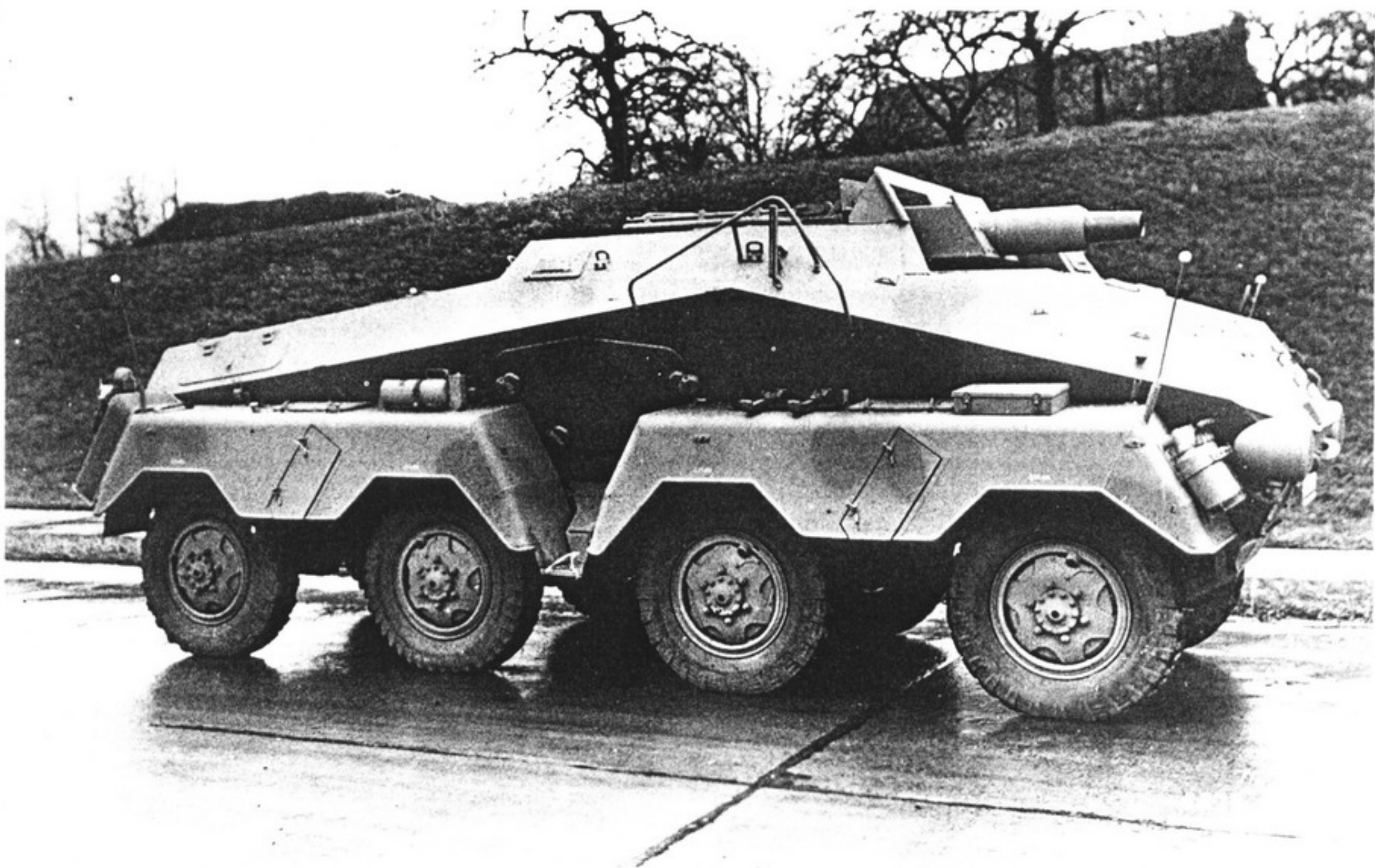
Above: A Sd.Kfz.233 with cast visors, completed in 1943, still has the Tropen (hot climate) camouflage pattern (NA)
