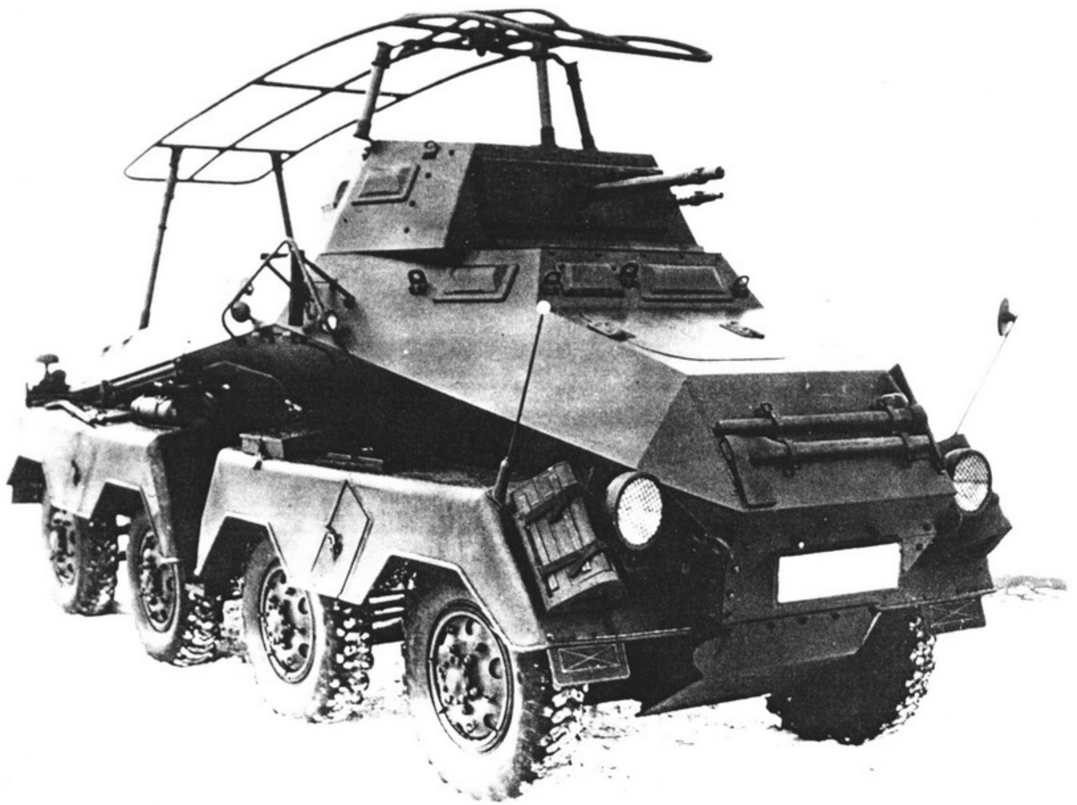
Above: A s.Pz.Sp.Wg. (Fu) (Sd.Kfz.232) with a frame antenna (WJS)
