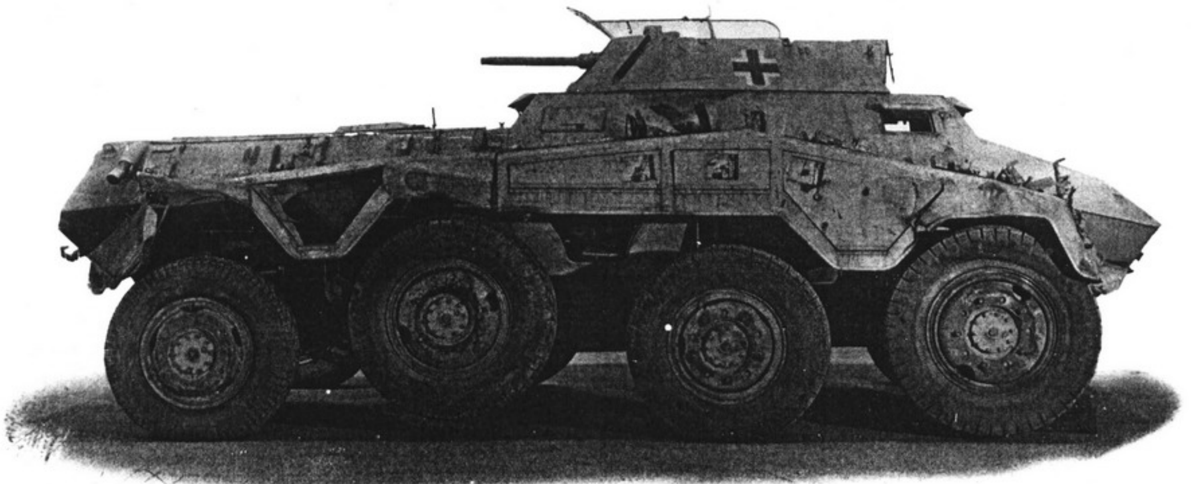
This Sd.Kfz.234/1, captured in Northwest Europe, had four stowage bins along the side (TTM)
