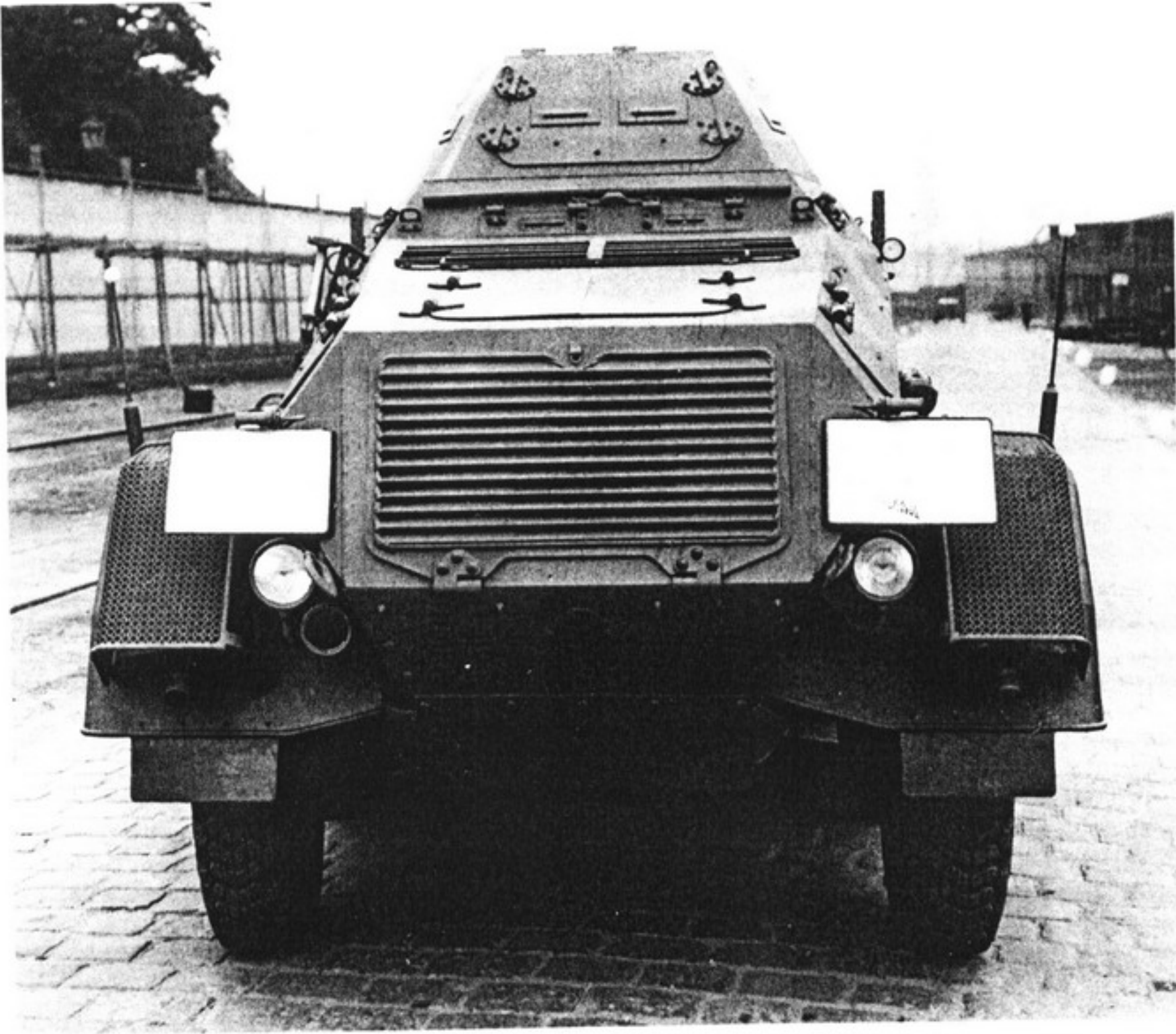
Left Above & Below: This s.Pz.Sp.Wg. (Sd.Kfz.233), completed in 1938 or early 1939, still has flat plate visors. (WJS)
