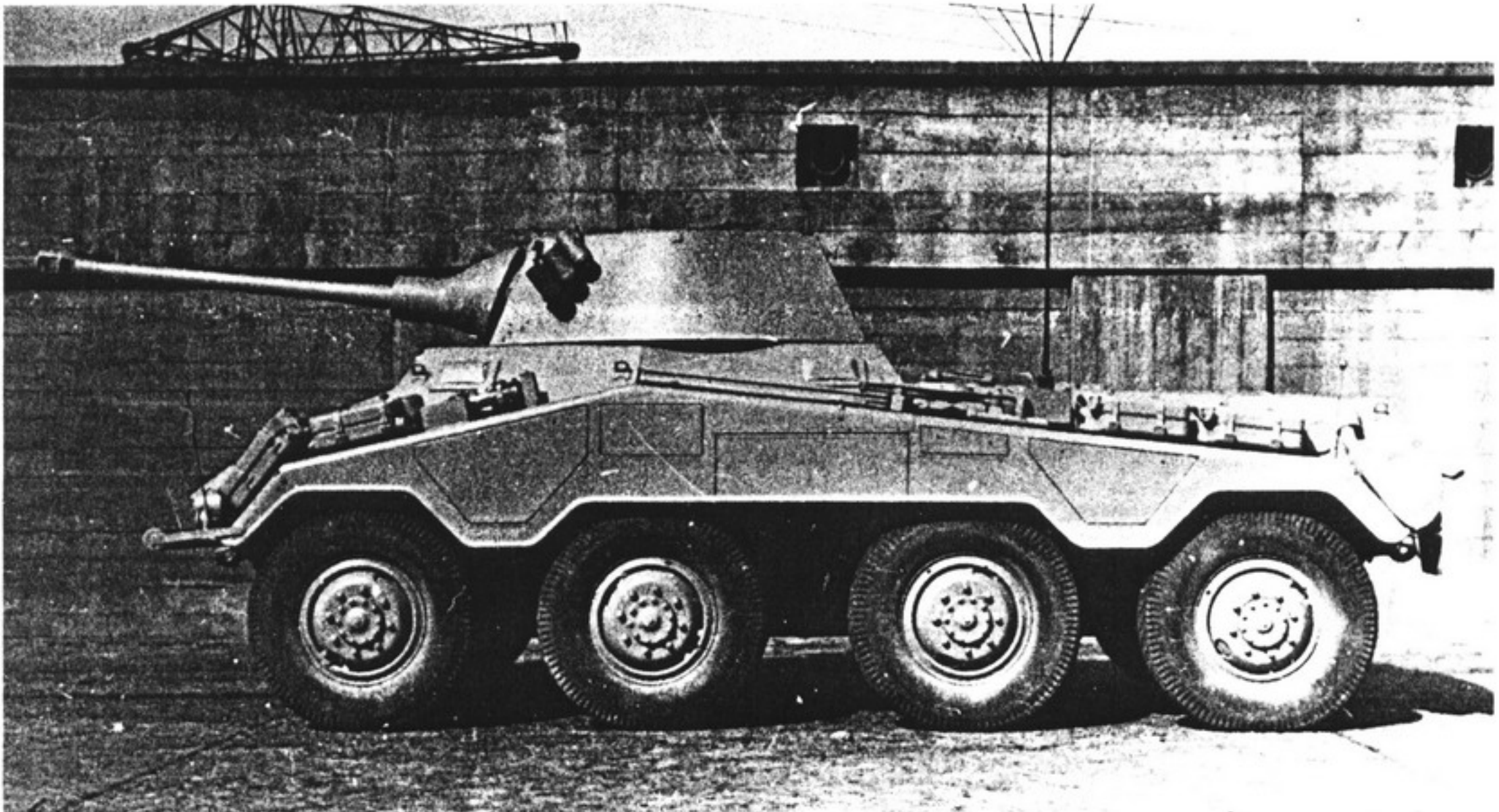
One of the first Sd.Kfz.234 with different pattern stowage bins completed in 1943 (NA)
