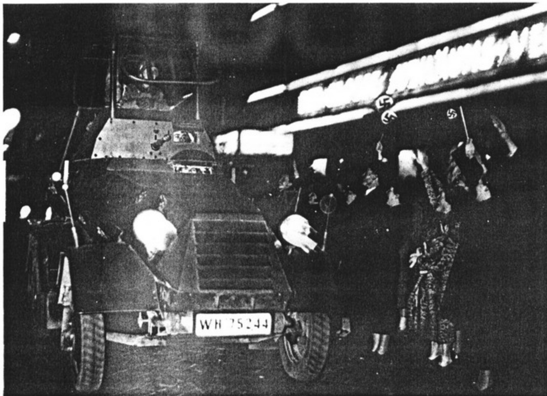
Right: One of the 12 Pz.Fu.Wg. (Sd.Kfz.263) (6 Rad) produced on Magirus M206a chassis. (WJS)
